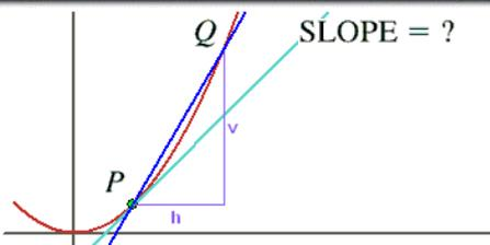
As  $Q$  approaches  $P$ , the slope of the secant  $PQ$  approaches the slope of the tangent at  $P$ .
